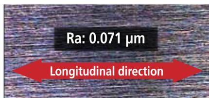
The quality of the slider bearing surface has improved due to use of the latest machining technology.
