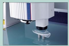
The Quick Vision Hybrid Type 4 is a machine which allows vision measurement with a CCD camera and high-speed scanning with a non-contact displacement sensor.
