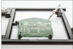
Support and clamping of a PCB at three points to enable positive location of the irregular profile at the measurement position.
