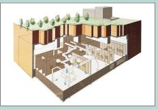
Mitutoyo's ultra-precision scale manufacturing facility eleven metres underground produces the exceptionally accurate scales for the Quick Vision Ultra.
