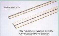
The Quick Vision Ultra is equipped with a crystallized glass scale having a resolution of 0.01  $\mu$ m and linear expansion coefficient of 0.08x10<sup>6</sup>/K. This virtually zero thermal expansion means the Quick Vision Ultra can minimize accuracy fluctuation resulting from thermal changes.
