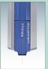
A stylus vibrating at an ultrasonic frequency enables the UMAP probe to sense contact with minute workpiece features. Five stylus tip diameters are available, from 15 to 300  $\mu m.$
