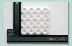
Batch measurement of identical parts simply located against connected rails.
