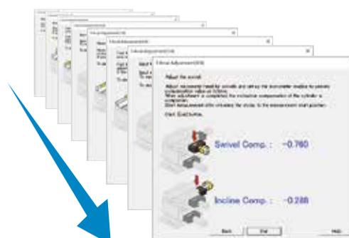
Guidance display when using 3-axis adjustment table
