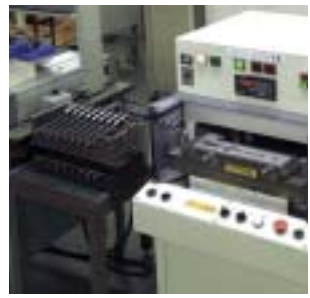
ABS Coolant Proof calipers being tested by air leakage test equipment
