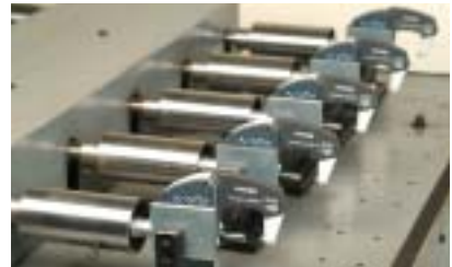
ABS Coolant Proof calipers being tested by air leakage test equipment
