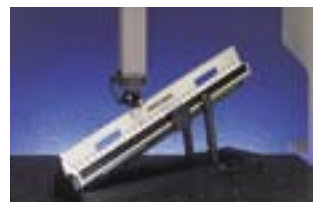
CMM calibration with Check Master No. 515-742
